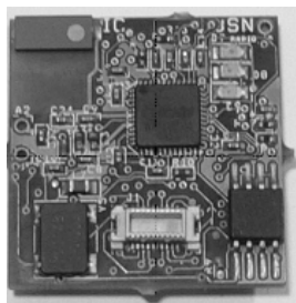
Figure A.9 A BSN node with a ceramic antenna.
