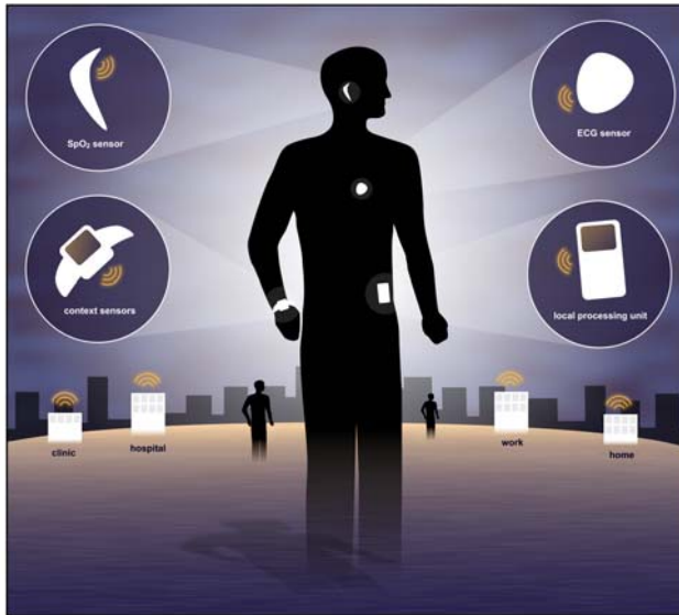
Figure 1.2 Diagrammatic representation of the BSN architecture with wirelessly linked context-aware “on body” (external) sensors and its seamless integration with home, working, and hospital environments. (See colour insert.)
